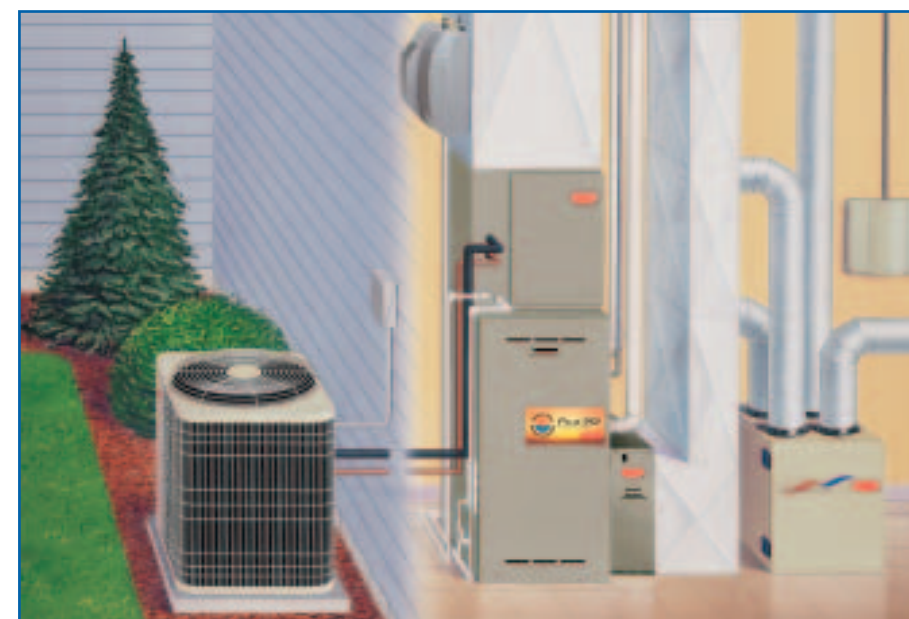
Central Air Conditioner and Gas Furnace System
